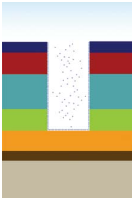
Figure 2. A post-clean via shows the presence of a monolayer of media and vapor that may be present in the via.
