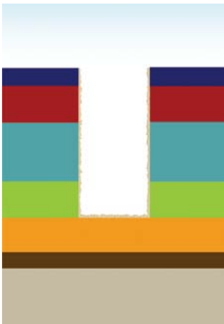
Figure 1. Illustration of a via structure following etching, with etch residue on sidewalls and floor of via.
