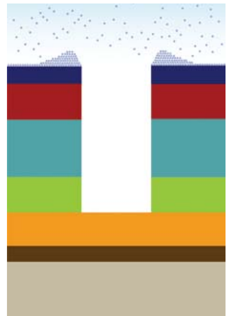
Figure 3. The scenario whereby residual media in the via "outgases" and deposits on the wafer surfaces adjacent to the via.
